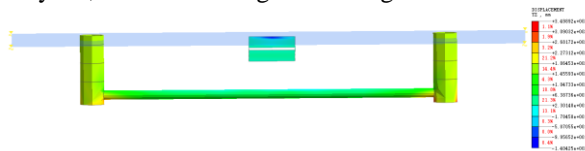
Figure 3. Settlement settlement of final construction
